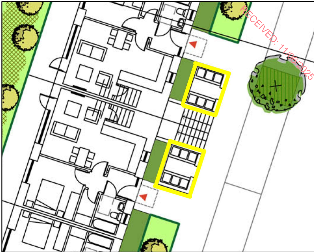
Figure 4-3 Internal layout of Waste Storage Areas in Block G1, G2, G3 and G4 (Yellow) (O'Mahony Pike, 2025)
