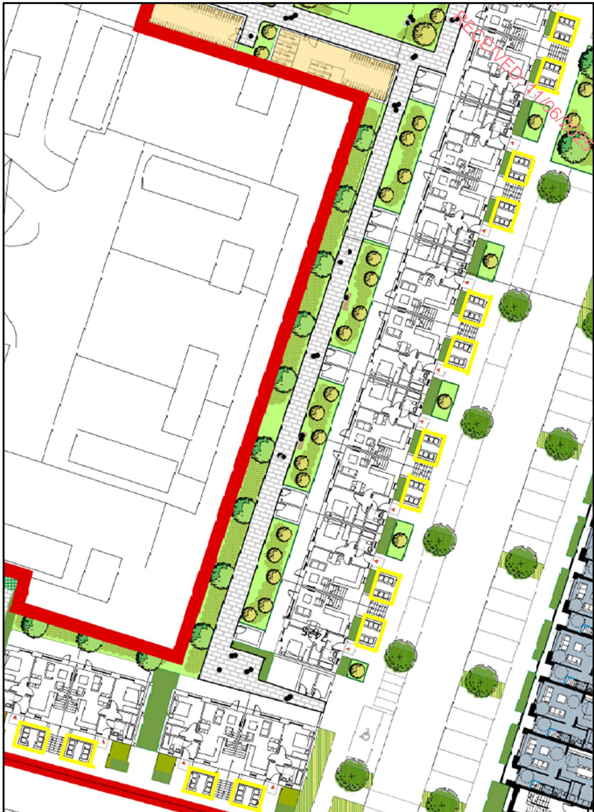
Figure 4-2 Location and internal layout of Waste Storage Areas in Block G1, G2, G3 and G4 (Yellow) (O'Mahony Pike, 2025)
