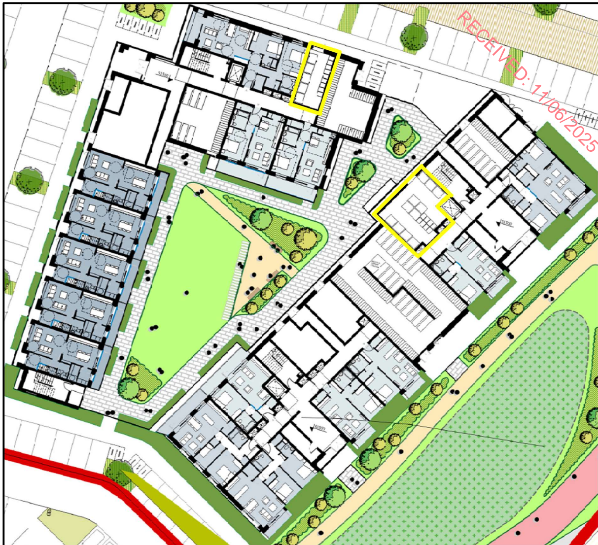
Figure 4-6 Location and internal layout of Waste Storage Area in Block E and F (Yellow) (O'Mahony Pike, 2025)
